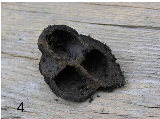
4 Remains of mud dauber wasp nest from end of tail pipe after decoking
